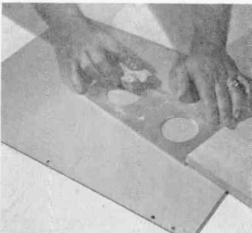
SANDING BLOCK corrects minor imperfections in both the metal and your workmanship. Use stopping block.
