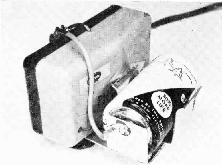
BATTERY , in its bracket is mounted behind one of the control units. When the relay closes, it applies this battery power to the small lamp, lighting the lamp and holding the relay closed. This takes the place and saves the cost of a latching relay.
